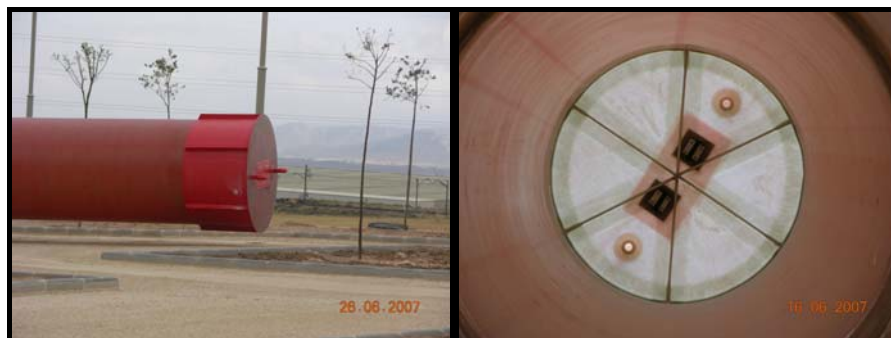
Fig. 6. External and internal details: flaps, pipes, sheaves and flanges.
