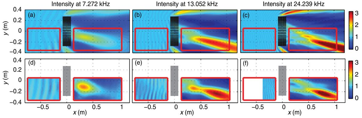
FIG. 4. Sound-pressure intensity in the vicinity of the lens at  $\omega a_x/2\pi c_b = 0.077$  (7.27 kHz), 0.138 (13.05 kHz), and 0.256 (24.24 kHz) for a source positioned at a  $15^\circ$  angle with respect to the  $x$  axis. (a)–(c) Pressure intensity calculated using 2D MST. (d)–(f) Measured pressure intensity. Gray boxes show the position of the lens. Red outlines indicate the experimentally mapped areas.
