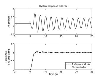
Figure 22: Closed-loop response with the neural network controller designed with 2 sensors and high-amplitude data
