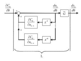
Figure 11: Sensitivity block diagram in open loop operation
