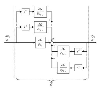
Figure 10: Block diagram of gradient propagation through the plant
