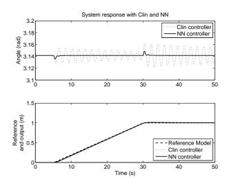
Figure 19: Comparison of plant behaviour with linear and neural network controllers (slow setpoint change speed)
