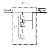
Figure 16: Tapped delay line of length x
