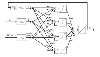
Figure 17: Neural network used for controllers of class  $C_2$
