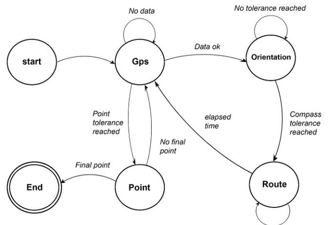
Fig. 2. AUV's states.
