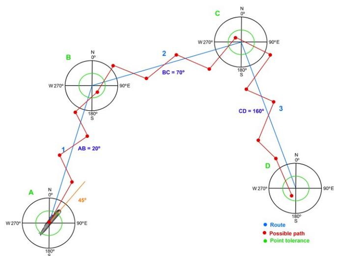
Fig. 3. AUV route example.
