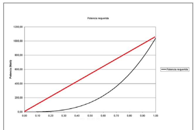
Fig. 15. Power-thrust function and linearization as upper limit
