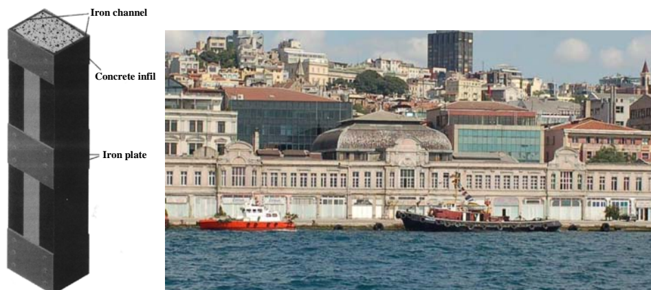
Figure 2: Galata Customs Building- column detail and façade
