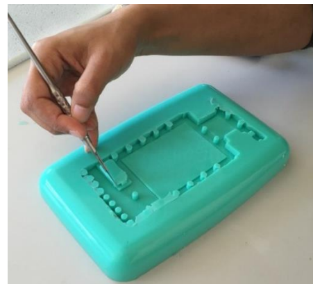
Figure 76 Cleaning of silicon mould
