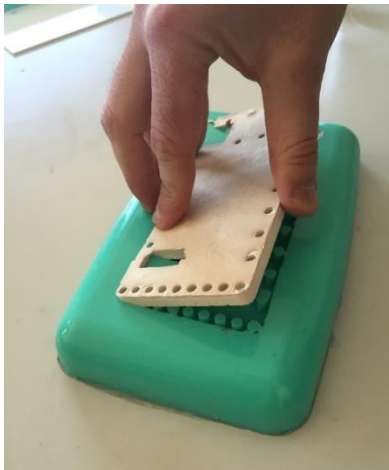
Figure 80 Moulded base out of mould
