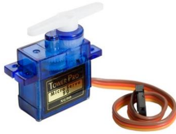
Figure 17 Micro servo for the arm
