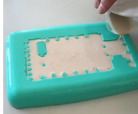
Figure 79 Setting acrylic resin
