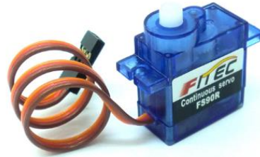
Figure 18 Continuous rotation servo for the wheels
