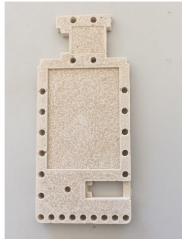
Figure 81 Acrylic resin base with broken edges
