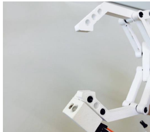
Figure 34 Colour sensor attached to the gripper
