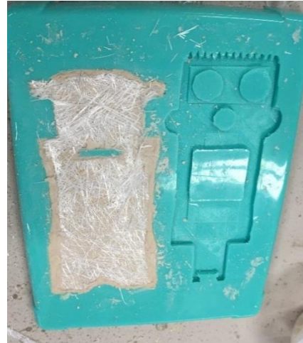
Figure 92 Glass fibre mat on the base
