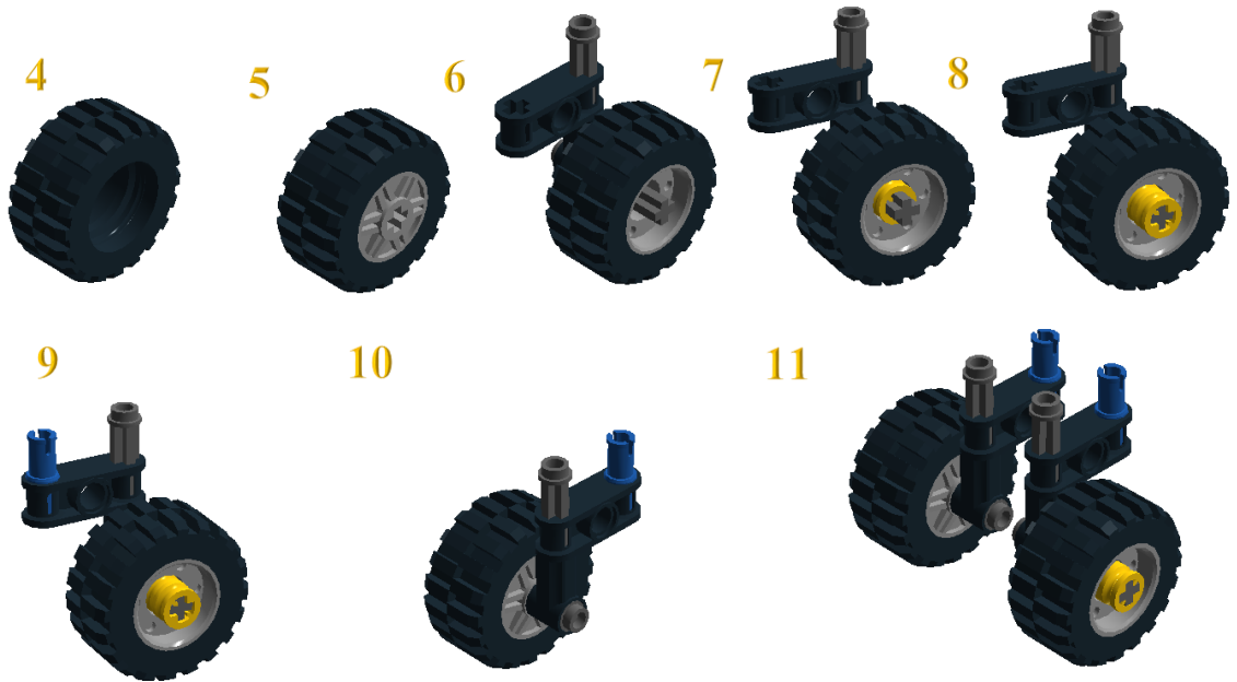
Figure 96 Steps to build front wheel arrangement 1
