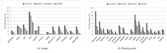
Figure 6. IPC degradation due to L2 contention
