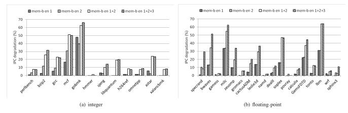
Figure 5. IPC degradation due to memory contention varying the number of co-runners
