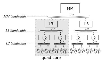
Figure 7. Contention points related to the memory subsystem in a three-level cache hierarchy CMP
