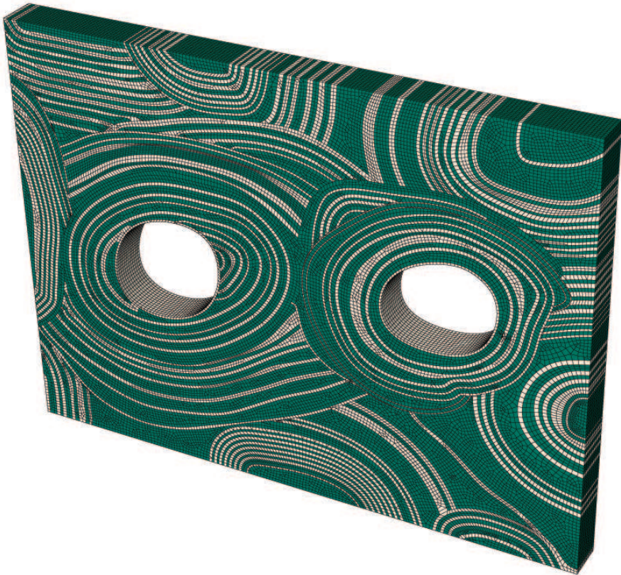
Figure 8.9: 3D FE mesh of the cortical bone micrograph with two osteons by Ebacher and Wang [2009]. The clear and dark colors show thick and thin lamellae.
