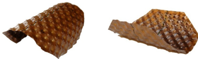
Figure 3: A doubly corrugated shell, showing anticlastic bistable behaviour.
