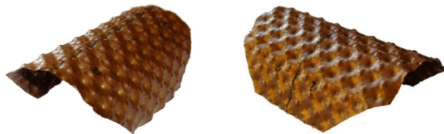
Figure 4: A doubly corrugated shell showing synclastic bistable behaviour.
