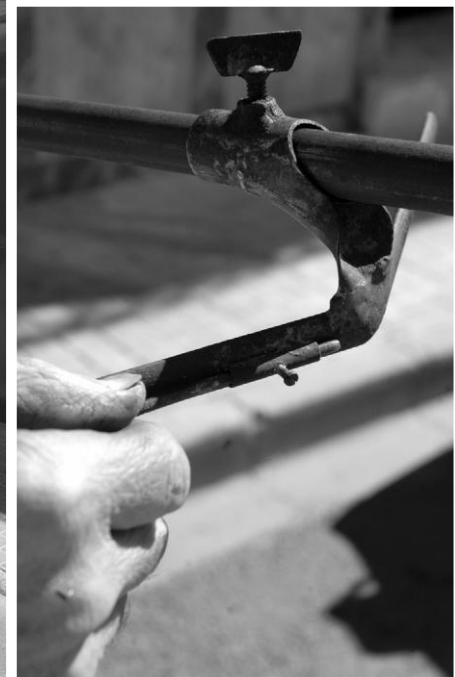
Figure 31. Detail of the sliding part of the instrument to build helical chimneys (Photo: author)
