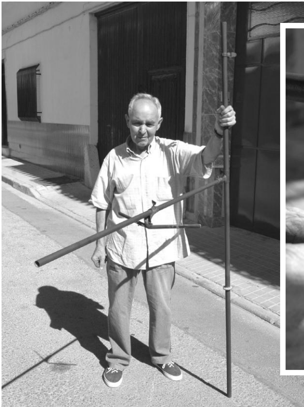
Figure 30. Antonio Jareño showing his invention for setting out helical octagonal chimneys (Photo: author)
