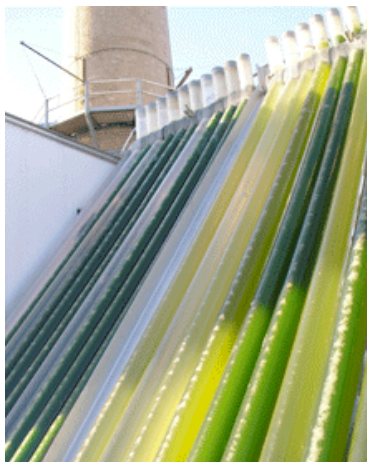
Figure 4 Smokestack emissions bubble through algae-filled tubes at MIT's Cogen plant. (Photo: Ashley Ahearn)
