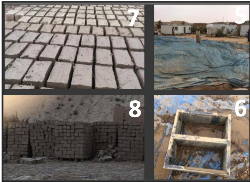
Figure 84. The process of making adobe in ad-Dirrya (Al-Aidarous,2013)
