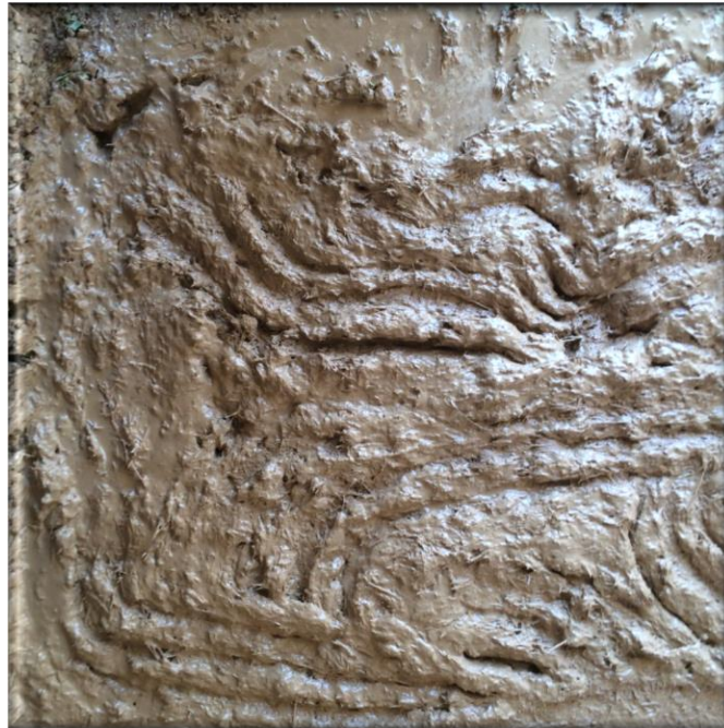
Figure 82. A mixture of earth with straw (Al-Aidarous)
