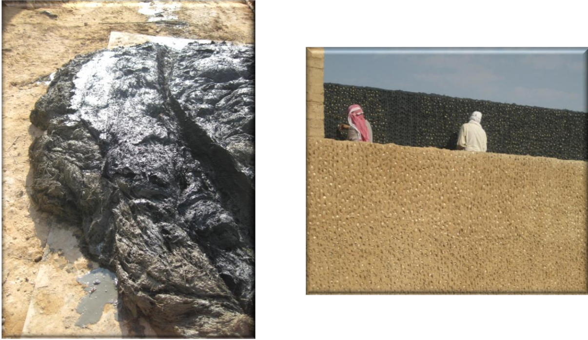
Figure 85. The resulting mixture used at ad-Dir'iyah for rendering and a mortar
