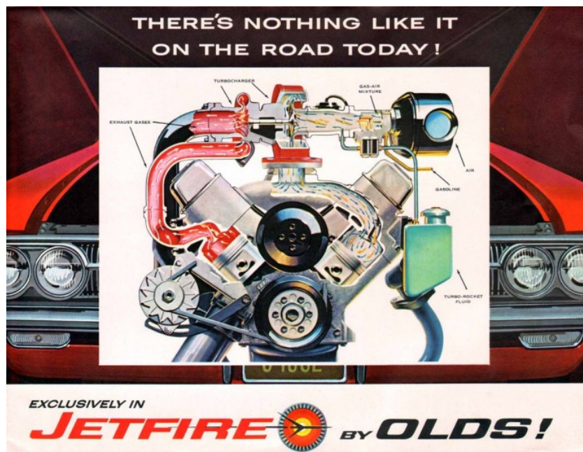
Figure 1.2. Advertisement of the 1962 Oldsmobile Jetfire, first mass production car with a turbocharged gasoline engine.
