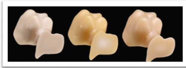
Figure 2.4 Zirconia tooth-shaped restorations with three different color shades after doping with other elements.
