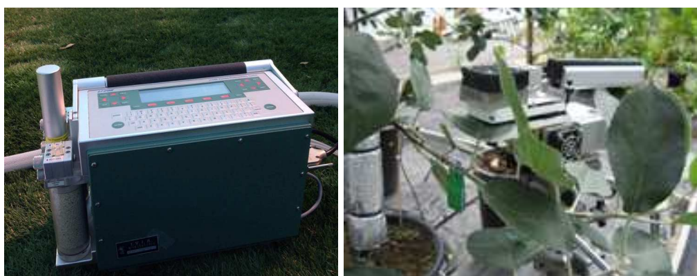
Figure 9. (left) Image of Li-cor 6400 portable photosynthesis system. The eggplant leaves were measured out of growth climatic chamber in the morning. (right) Illustration when the leaves were measure using Li-cor 6400 portable photosynthesis (the eggplants leaves measurement was not recorded).
