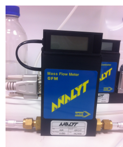
Figure 6. Air Mass Flow Meter (GFM).
