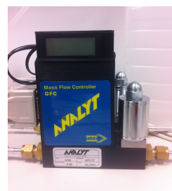
Figure 7. CO 2 Mass Flow Controller (GFC).
