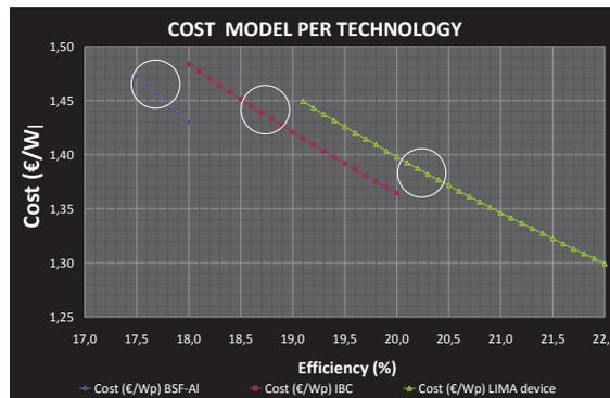
Fig. 8. Module cost in €/Wp versus solar cell efficiency per technology. Threshold efficiency at solar cell level are shown for IBC technology (18.5%) and for LIMA technology (20%).
