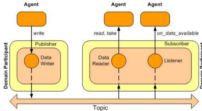
Fig. 1. Overview DCPS components from the DDS model.
