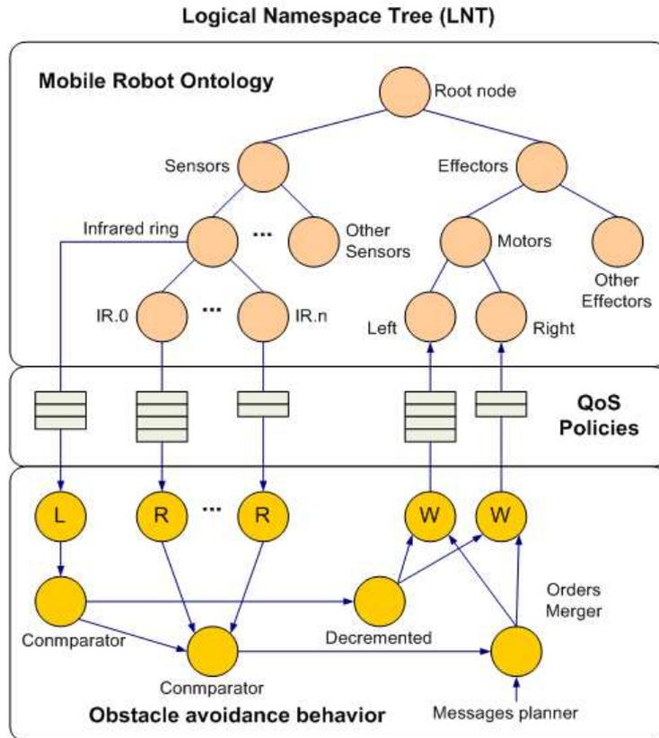
Fig. 5. Example of ontology to provide information to a obstacle avoidance behaviour.
