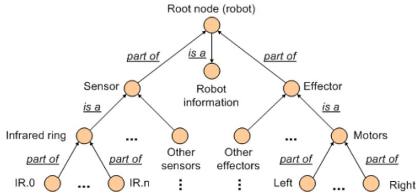
Fig. 3. Example of mobile robot system ontology.
