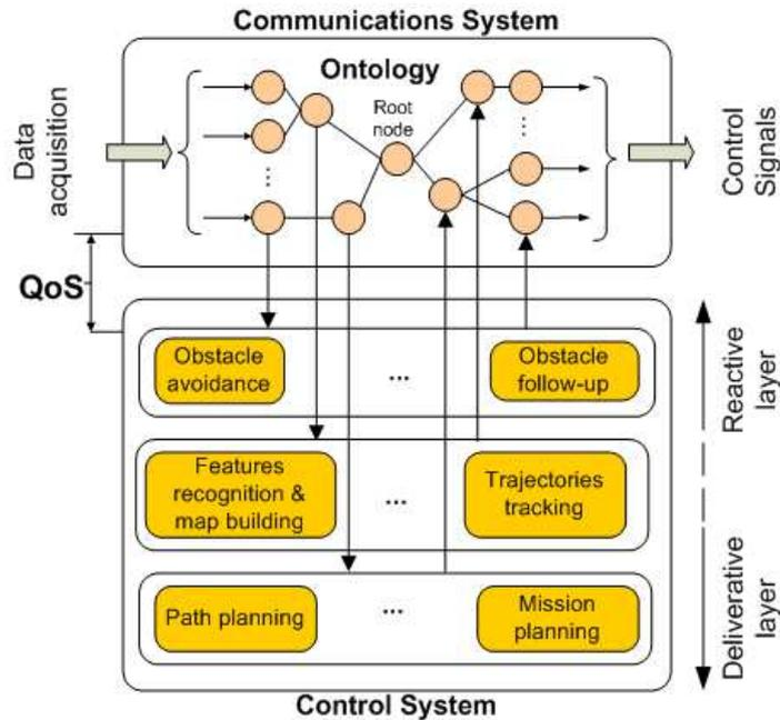
Fig. 4. Robot navigation architecture implemented with the FSA-Ctrl architecture.
