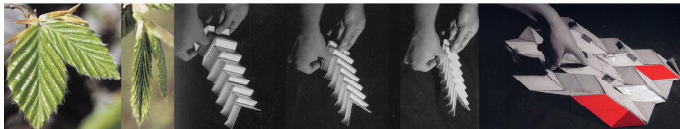
Figure 14: Extrapolation of the geometry of the beech leaf to a deployable roof (Lim)
