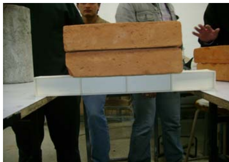
Figure 9a. Test that shows the resistance of the beam under uniform load.
