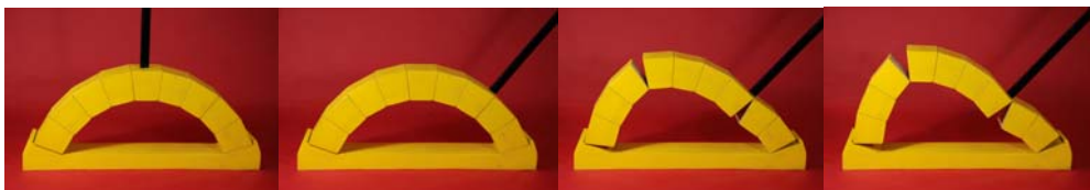
Figure 6. Keystone arch. Deformation under different types of loads.
