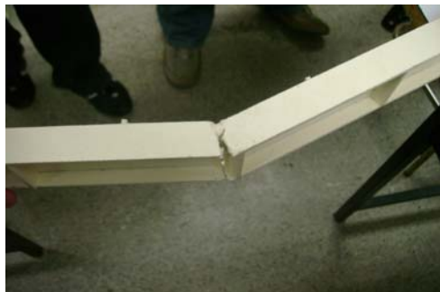
Figure 9b. In this picture we can appreciate the beam breaking.
