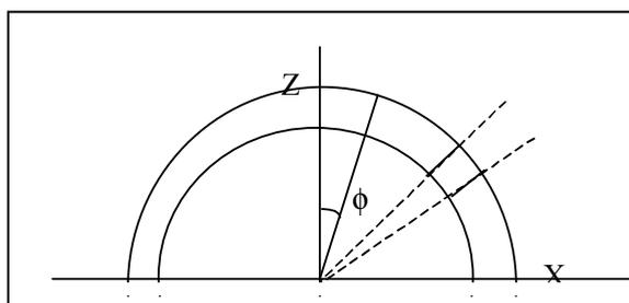
Figure 10: Section parallel to the XZ-face. For the meridians the angles  $\phi$  of the normal lines with the Z-axis do not vary.
