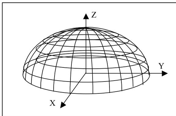
Figure 1: The globe-grid. The meridians are jointed at the top and the parallels are ellipses constructed in faces parallel the ground face.
