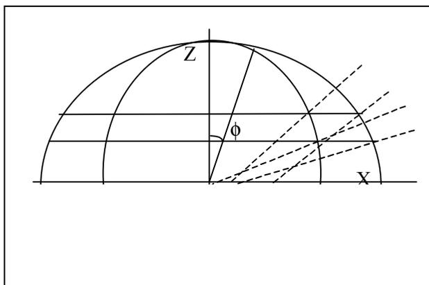
Figure 4: The normal lines drawn for four points of the surface projected on the X-Z face.
