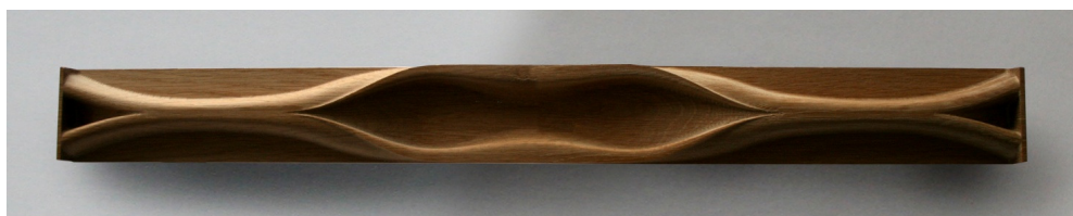
Figure 5: CNC-milled model of optimised slab.
