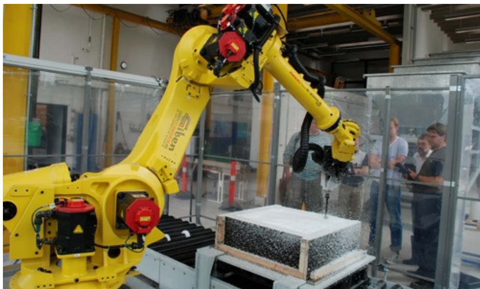
Figure 14: Large Scale CNC-milling robot at the High Technology Concrete Workshop at the Danish Institute of Technology
