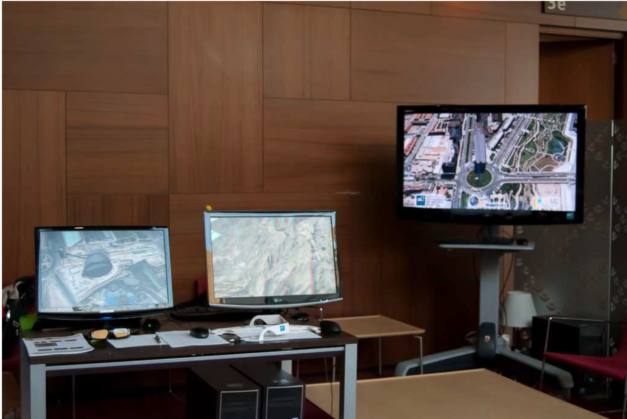
Figure 6: Equipments used for the test, all of them running on full screen option in order to enhance the illusion of depth. From left to right: quadbuffer system, anaglyphs and autostereoscopic screen with lenticular filter.
