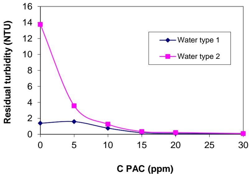
Figure 5. Results for Jar test with water type 1 and water type 2
