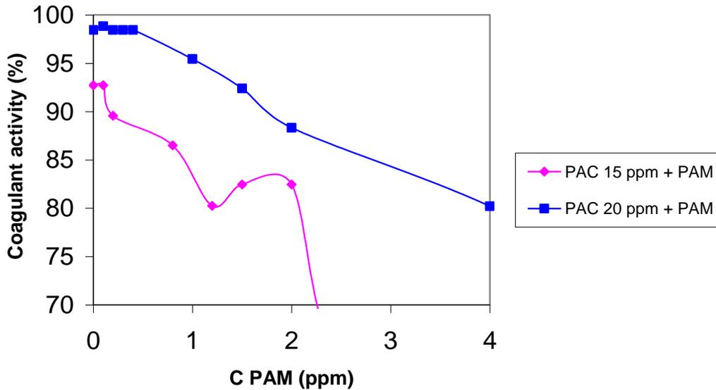
Figure 4. Results of Jar test using PAC and PAM in type 1 water
