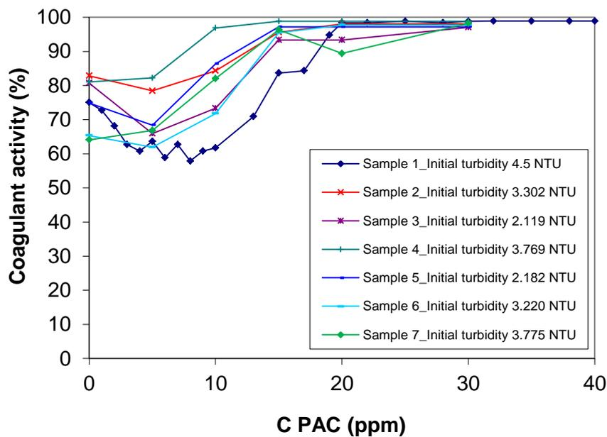
Figure 2. Results of Jar test using PAC as coagulant with type 1 water
