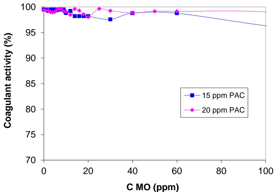
Figure 7. Jar test results for water type 2, using PAC as coagulant and a MO as coadjuvant
