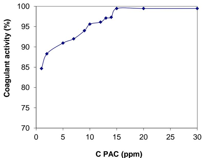
Figure 6. Jar test results for type 2 water, using PAC as coagulant and 0.3 ppm of PAM
