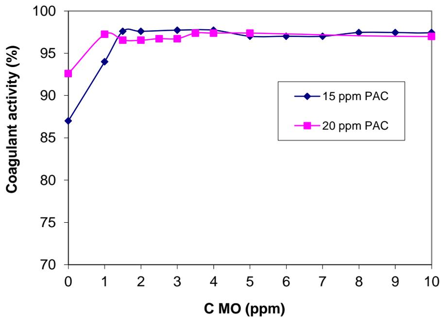
Figure 3. Results of Jar test using PAC and *Moringa* in type 1 water
