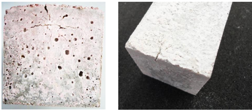
Figure 12-4 Two photos showing cracking damage at the impact location.
