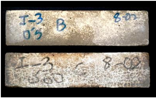
Figure 8-4 Surface of mortar samples I-050 (above) and I-060 (below) after 5 freezing-thawing cycles. Prismatic samples measuring 4 \times 4 \times 16 \text{ cm}^3 .
