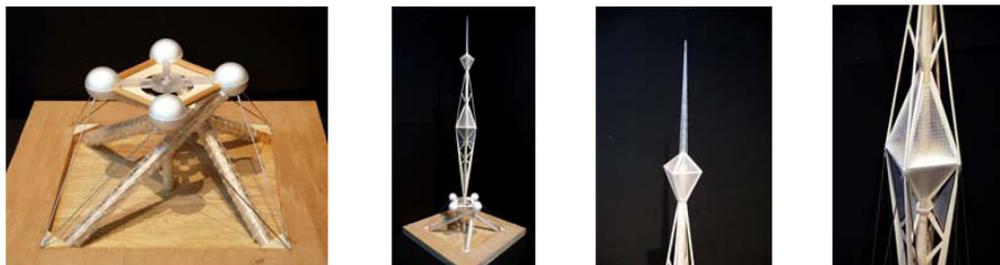
Figure 12: Modelling process for structural system
