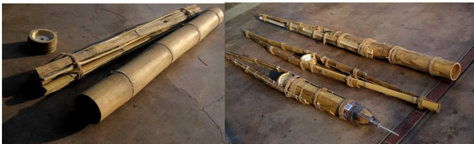
Figure1. Analogue Modulation: Diaphragms section, laminated sections and rolled sections and (left) The generatrix Unit (The identity) and possibilities (right) – Bamboo-flex Mechanism.
