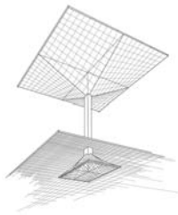
Figure 4: Candela’s umbrellas: A sketch showing straight lines generating the surface and Rio’s warehouse (right) under construction.
