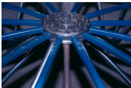
Figure 2 Connection types by bolt with gusset plate in test model (A)
