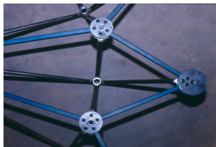
Figure 2 Connection types by bolt with gusset plate in test model (A)
