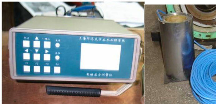
Figure 7: EM sensor and voltage oscillograph
