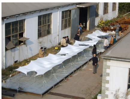
Figure 4: Pre-stressed initial state of the model
