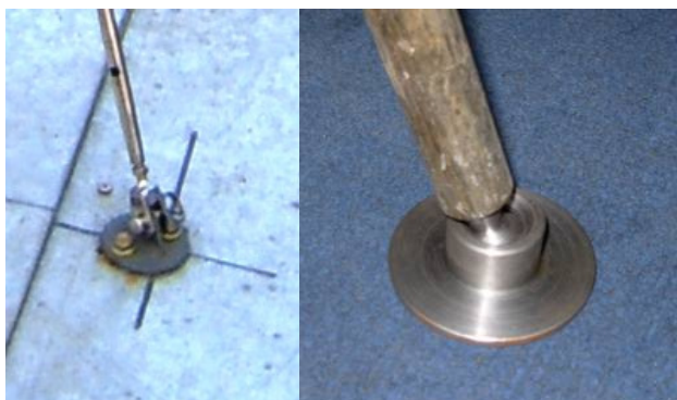
Figure 3: Pin-joints of the ends of cables and masts in test model
