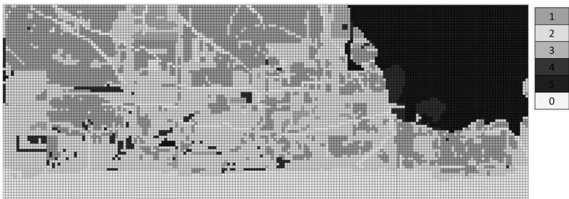
25 26 Fig. 4 Damage mapping of Wall 4 (facing to the north) of room 2. Legend of equivalence between the 27 grey scale and numerical scale of damage stages is represented
