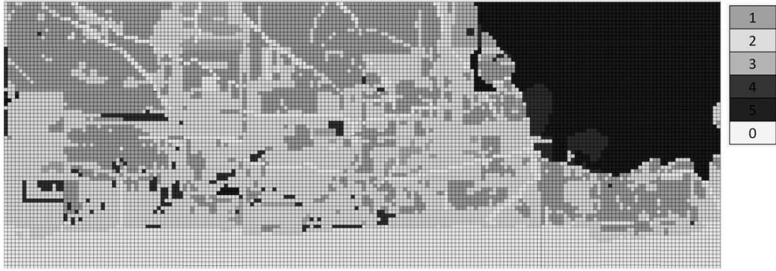
2 Fig. 4 Damage mapping of Wall 4 (facing to the north) of room 2. Legend of equivalence between the 3 grey scale and numerical scale of damage stages is represented
