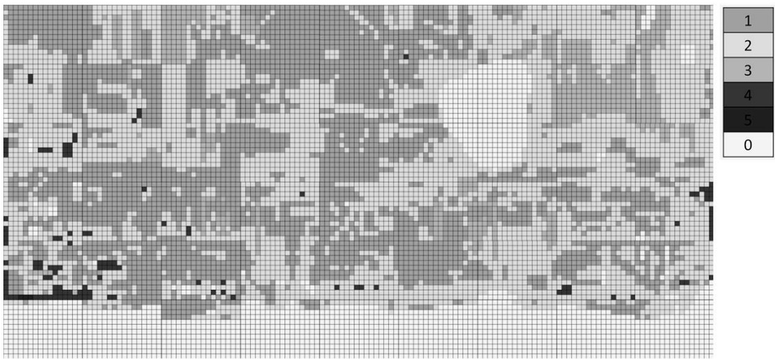
2 Fig. 4 Damage mapping of Wall 4 (facing to the north) of room 2. Legend of equivalence between the 3 grey scale and numerical scale of damage stages is represented
