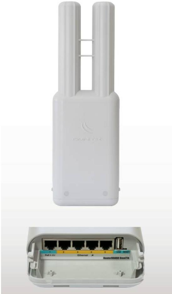
OmniTIK is a weatherproof outdoor AP with dual-polarized omni antennas - the perfect companion for our SXT, or for any other 5GHz 802.11a/n standard device.
