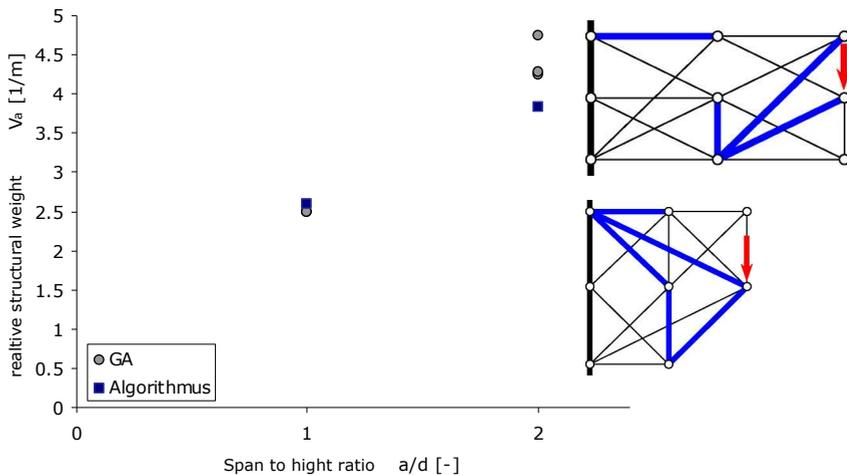
Figure 8: Comparison between the structural weight of the topology optimized truss structures using the presented topology optimization algorithm and a genetic algorithm
