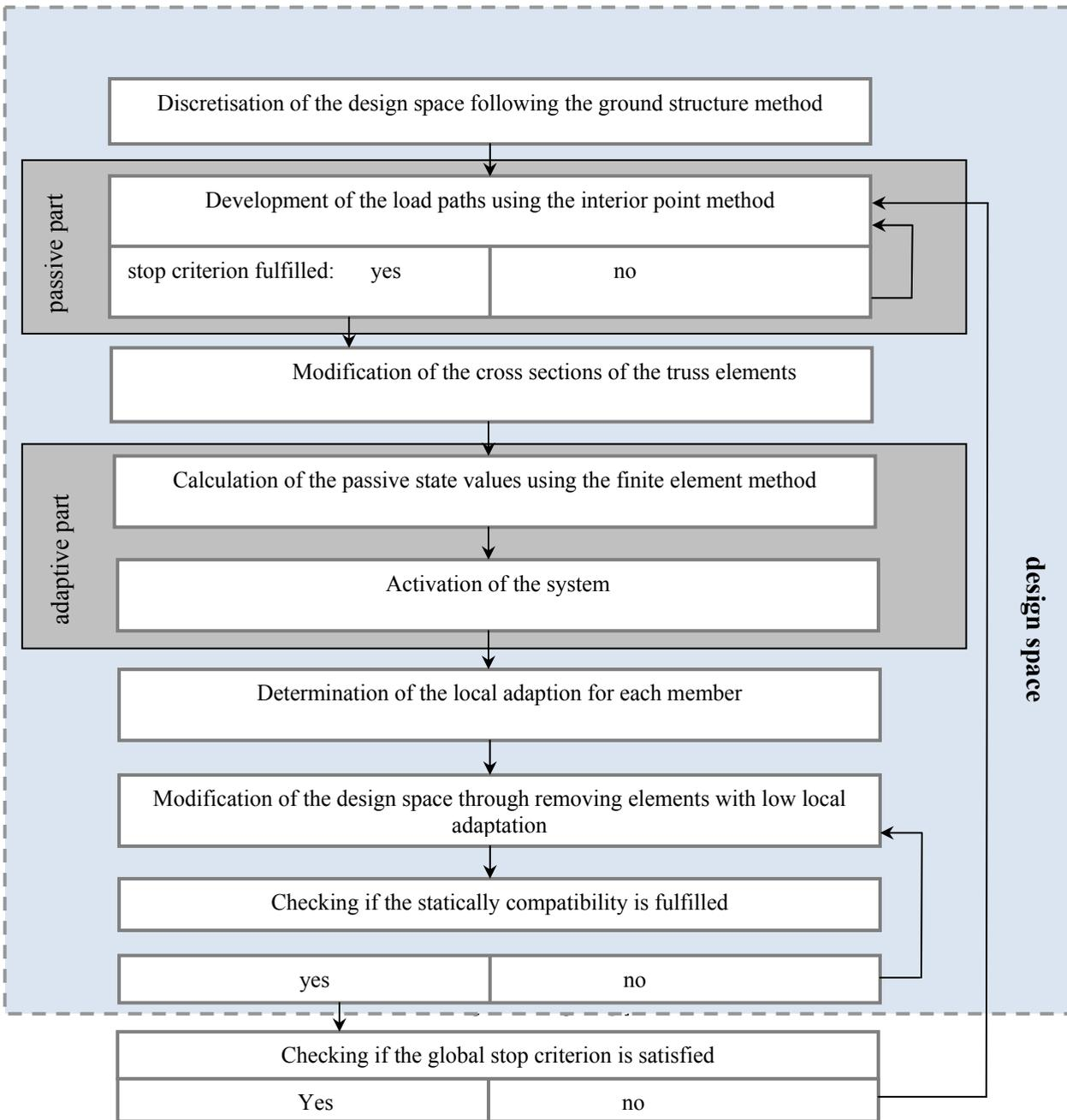
Figure 3: scheme of interaction of the adaptive and the passive part of the topology optimization algorithm
