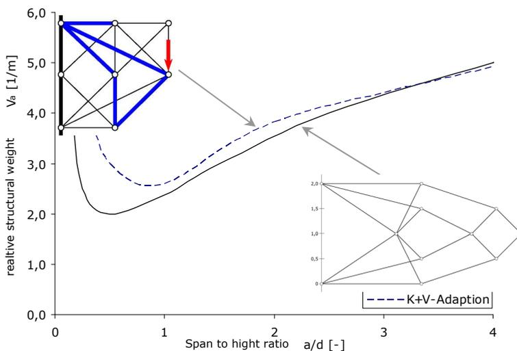
Figure 5: Comparison between the structural weight of Michell-Structures and the topology optimized adaptive truss structures under simultaneous force and deformation adaptation and single load case
