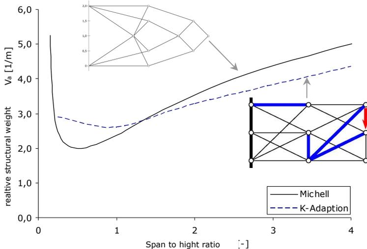
Figure 4: Comparison between the structural weight of Michell-Structures and the topology optimized adaptive truss structures under simultaneous force and deformation adaptation and a single load case
