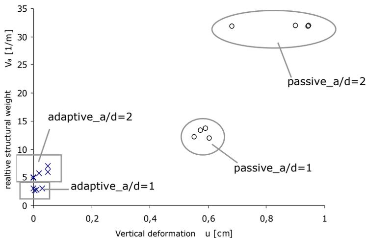
Figure 6: Comparison between the structural weight of Michell-Structures and the topology optimized adaptive truss structures under simultaneous force and deformation adaption and multiple load cases
