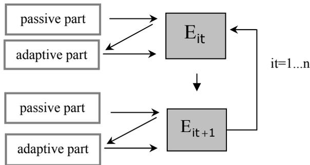
Figure 2: scheme of interaction of the adaptive and the passive part of the topology optimization algorithm
