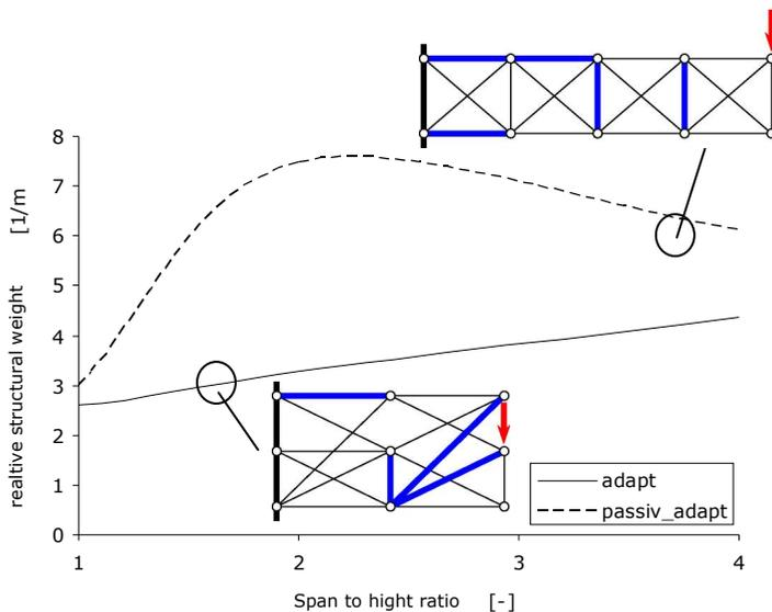
Figure 7: Comparison between the structural weight of the topology optimized adaptive truss structures and conventional adaptive truss structures
