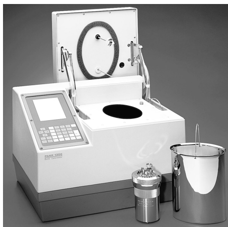
Figure 3.16: Calorimeter used to evaluate the Q_{HV} of the diesel fuel during the fleet test.
