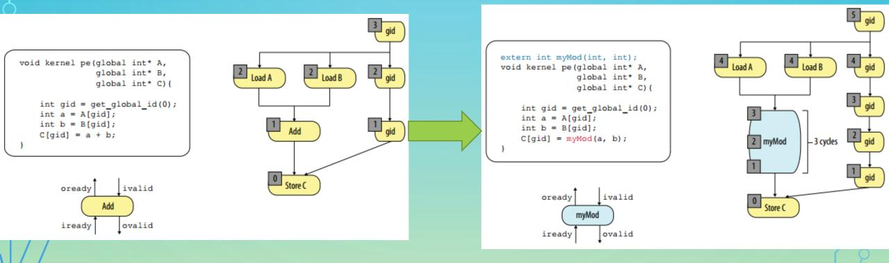
Parallel Execution Model of AOCL Pipeline Stages Integration of an RTL Module into an AOCL Pipeline
