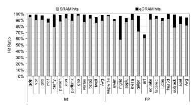
**Fig. 2.** Hit ratio (%) split into SRAM and eDRAM hits per benchmark for the HER cache in *hp* mode.
