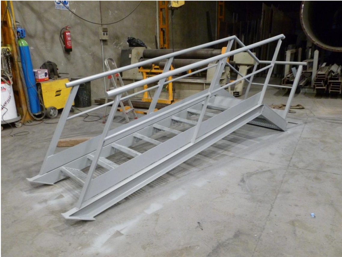
Service stairs for a silo
