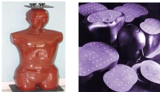
Figure 1. RANDO laboratory phantom.
