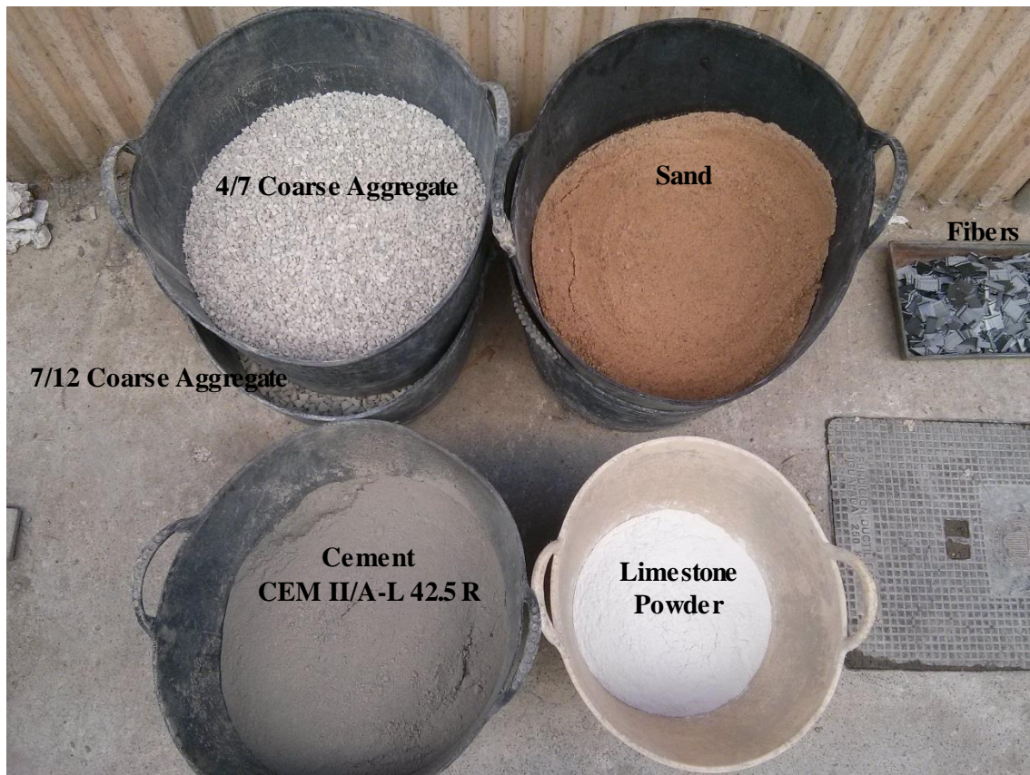
Fig. 3-2 – Main compounds used for casting concrete.
