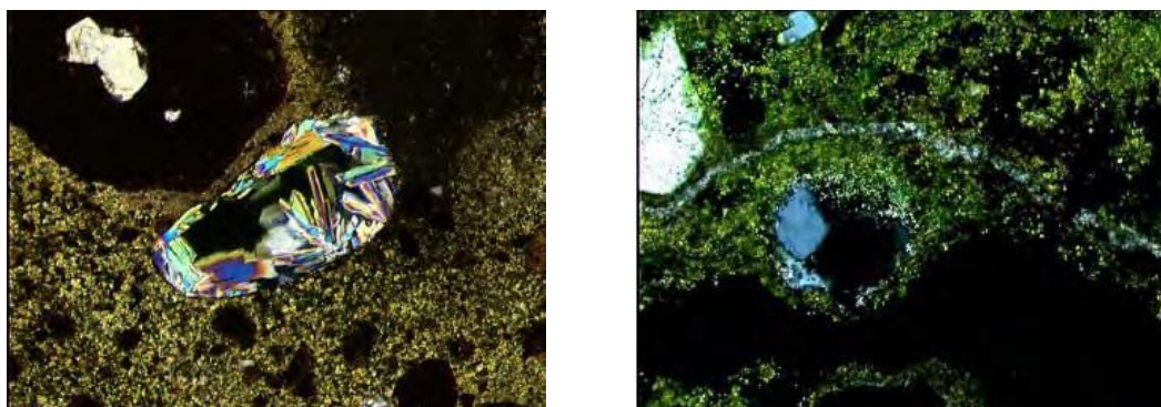
Fig. 2-8 - Microphotograph showing large portlandite crystals in air void in early 19th century lime (left) and a crack filled completely by calcite (right) (Nijland, et al., 2007).
