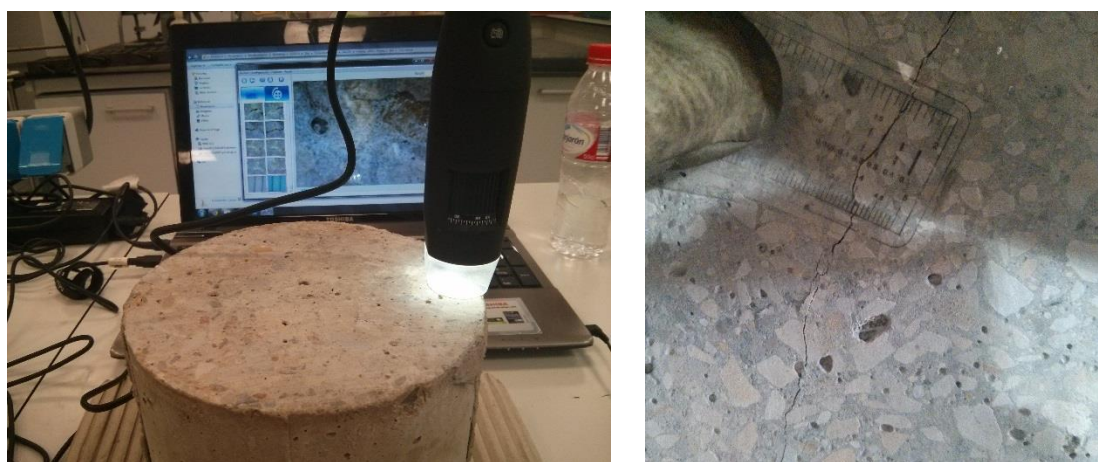
Fig. 3-16 – Optical microscope connected (left) and crack width ruler (right).
