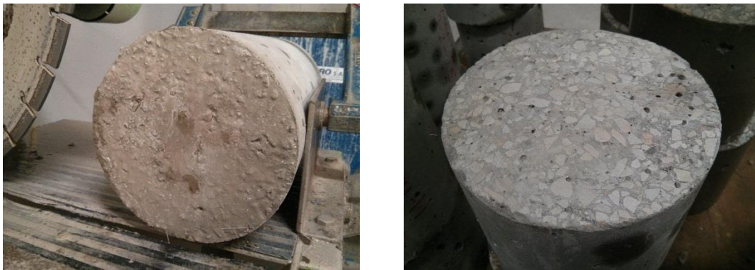
Fig. 3-10 – Irregular surface before polishing with the circular saw (left) and final aspect (right).
