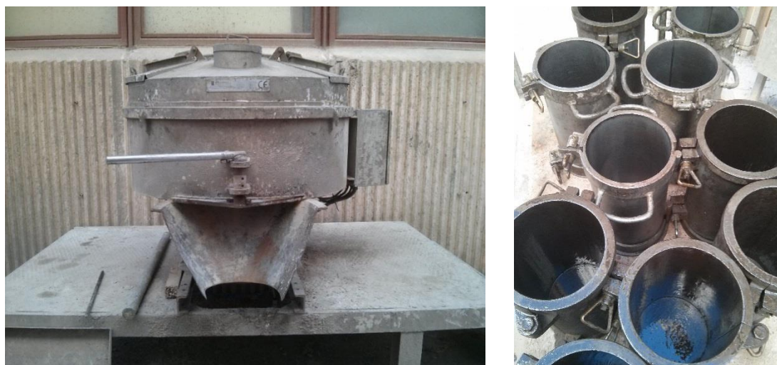
Fig. 3-5 –Planetary mixer used for casting concrete (left) and cylindrical molds (right).
