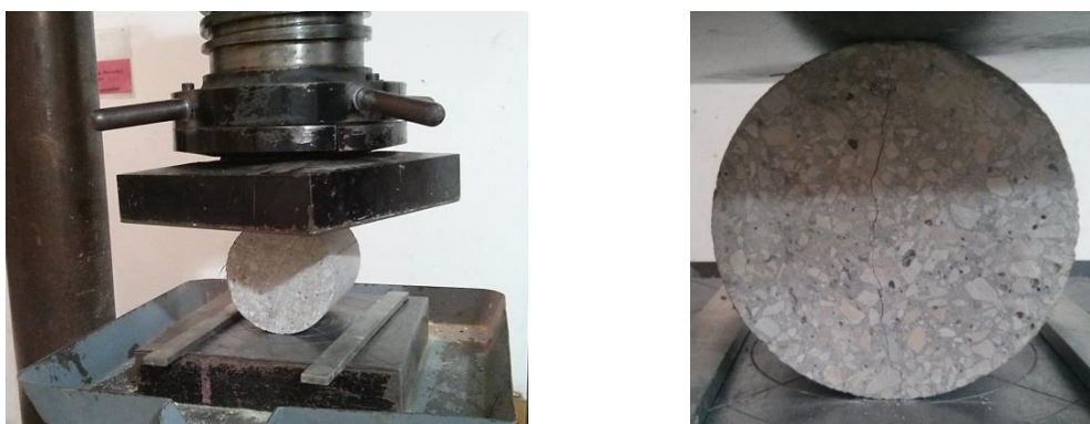
Fig. 3-11 – Pre-cracking process and pre-cracked specimen by splitting test.
