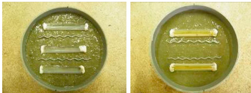
Fig. 2-47 – Glass tubes with bacterial solution are added to mortar disks analogously to steel reinforcement (Wang, et al., 2012).
