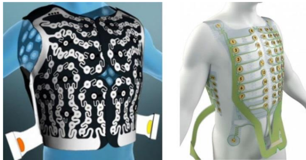
Figure 2.11 – Body surface potential mapping systems. Two examples of electrode distribution for BSPM recording.
