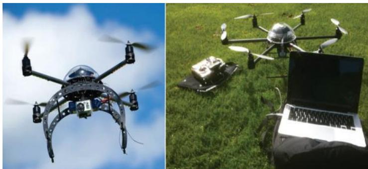
Figura 15. HexaKopter and QuadKopter (Van Bueren and Yule, 2013)
