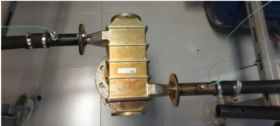
Figure 4.15. Heat exchanger on the test bench
