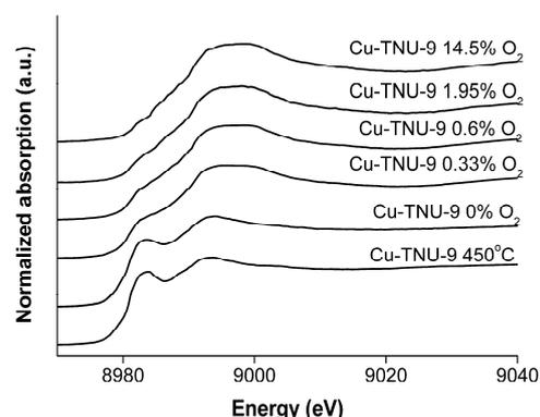
**Figure 2.** Cu K-edge XANES spectra of Cu-TNU-9 obtained under catalytic conditions ( $T= 450\text{ }^{\circ}\text{C}$ ; 700 ppm NO and 390 ppm C<sub>3</sub>H<sub>8</sub> balanced in He) and at different O<sub>2</sub> concentrations (0-14.5 %).
