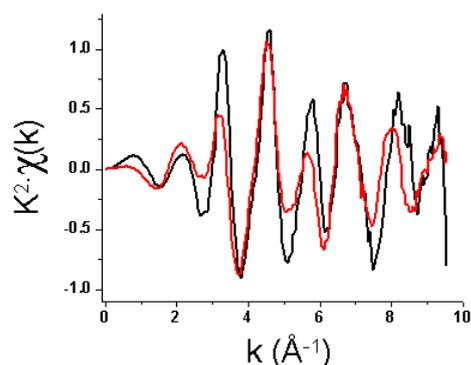
**Figure 6.** k<sup>2</sup> weighted EXAFS signal obtained in transmission at the Pd K-edge before (black) and during (red) the selective hydrogenation of the cinnamaldehyde by 2 wt% Pd/Sn-Beta zeolite catalyst.
