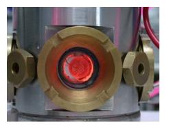
**Figure 3.** External view of the in-situ cell while heating the sample at  $700^{\circ}$ C.
