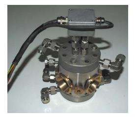
**Figure 1.** External view of the multipurpose in-situ cell for solid-gas catalysis.
