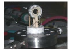
**Figure 4.** Internal view (upside down) of a prototype of half electrochemical cell
