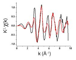
**Figure 6.**  $k^2$  weighted EXAFS signal obtained in transmission at the Pd K-edge before (black) and during (red) the selective hydrogenation of the cinnamaldehyde by 2 wt% Pd/Sn-Beta zeolite catalyst.
