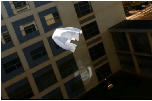
Fig. 13. Test of the rocket recovery system
