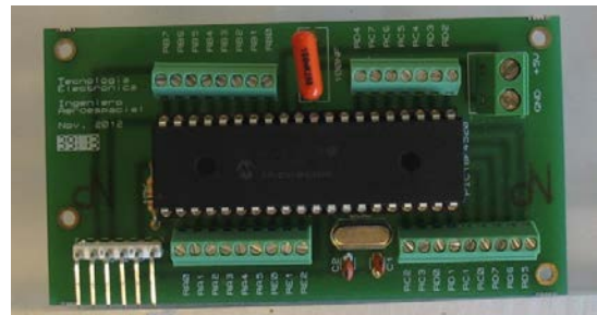
Fig. 3. Home-designed PCB with PIC18F4520
