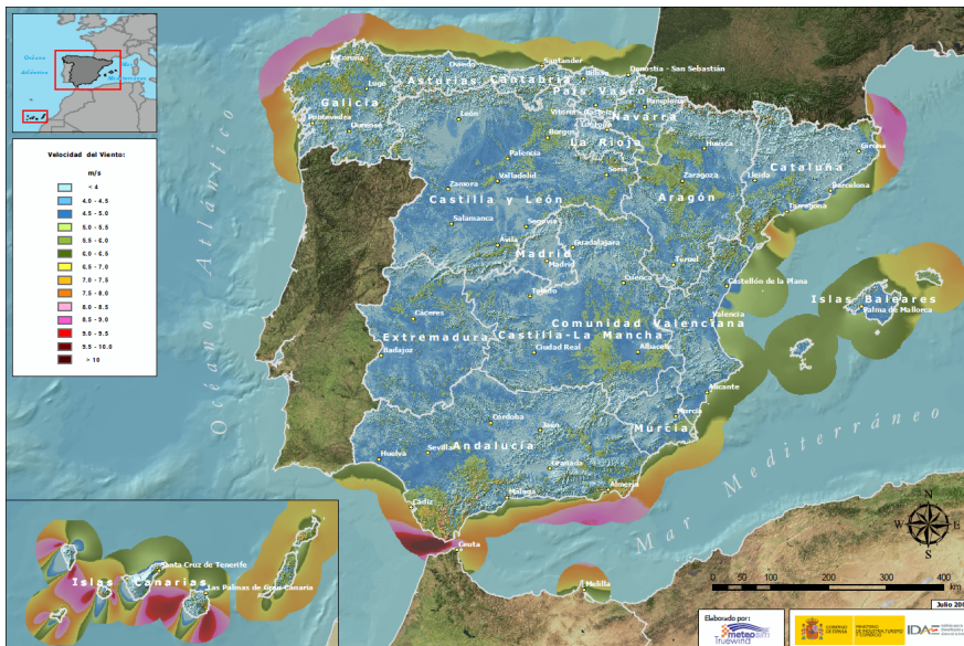
Figure 2.11: Average Speed at 30 meters height in Spain.
