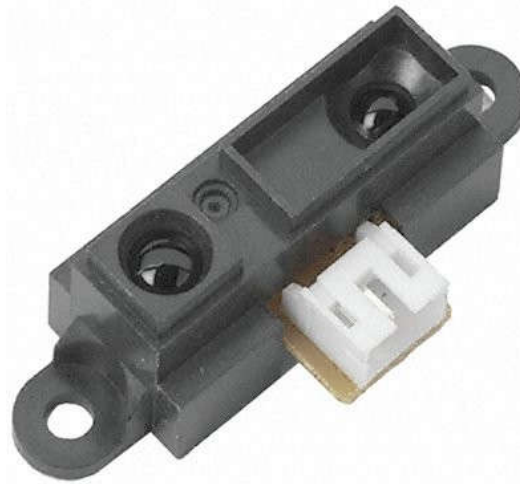
Illustration 5. Sharp GP2Y0A21YK. (Sharp n.d.)
