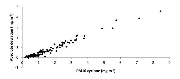
Figure 3. Absolute deviation (mg m<sup>-3</sup>) between DustTrak and cyclone sampler for poultry and pig dataset (n= 112, excluding turkeys), as a function of PM10 concentrations measured with cyclone sampler.
