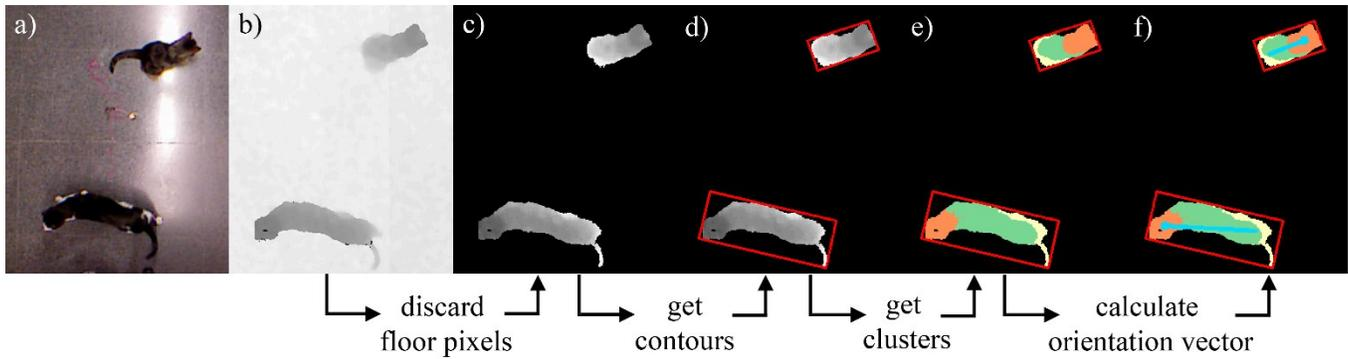
**Figure 2.** Process of extracting the cat's orientation: (a) color frame (b) depth frame, (c) background segmentation, (d) cat contours, (e) clusters for head, body and tail, (f) orientation vector
