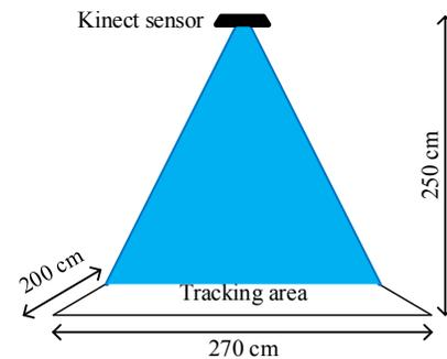
Figure 1. Set up for the tracking system
