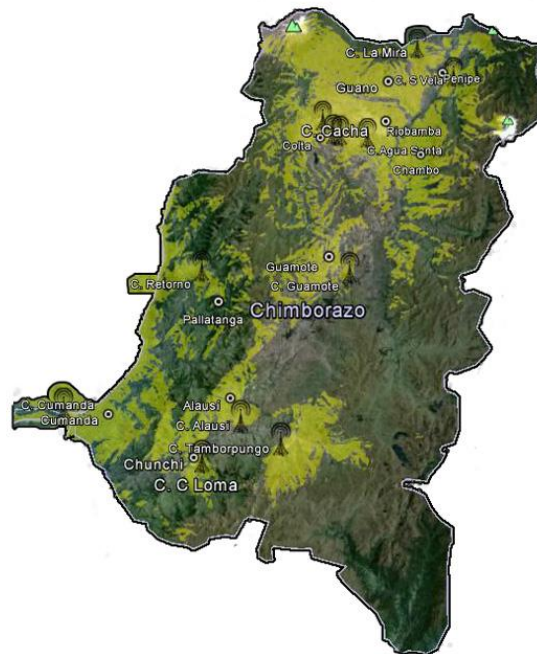
Figura 5. Cobertura UL DVB-RCT2 MODCOD QPSK \frac{1}{2} .
